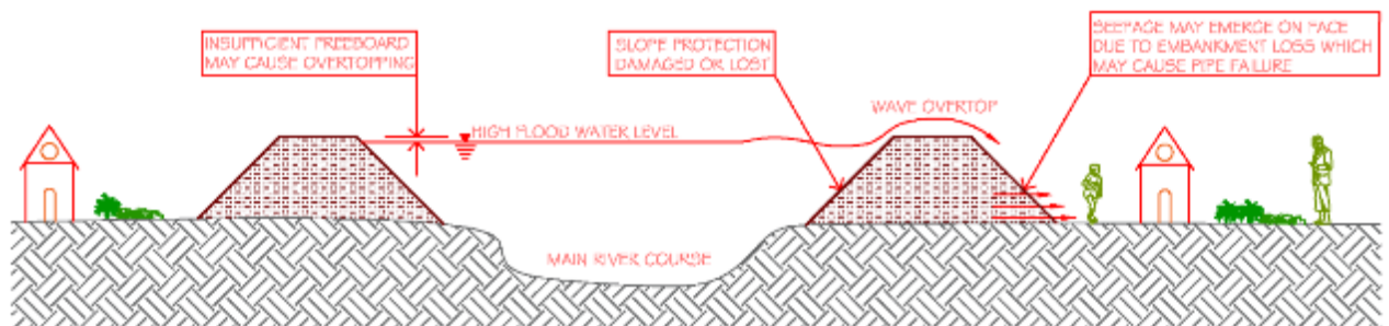
Figure 10: Issues of Existing River Embankment Requiring Rehabilitation
